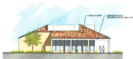
SOUTH ELEVATION BLDG. C SCALE 1/16"=1'-0"
