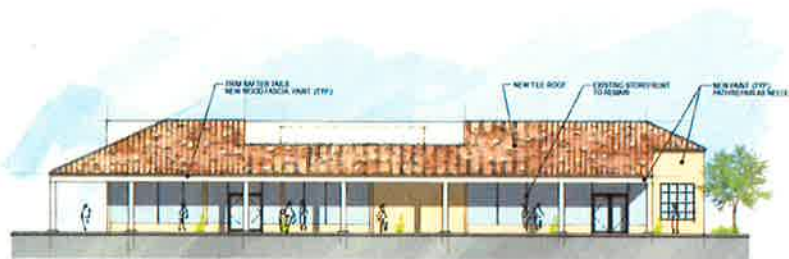
EAST ELEVATION BLDG. C SCALE 1/16"=1'-0"
