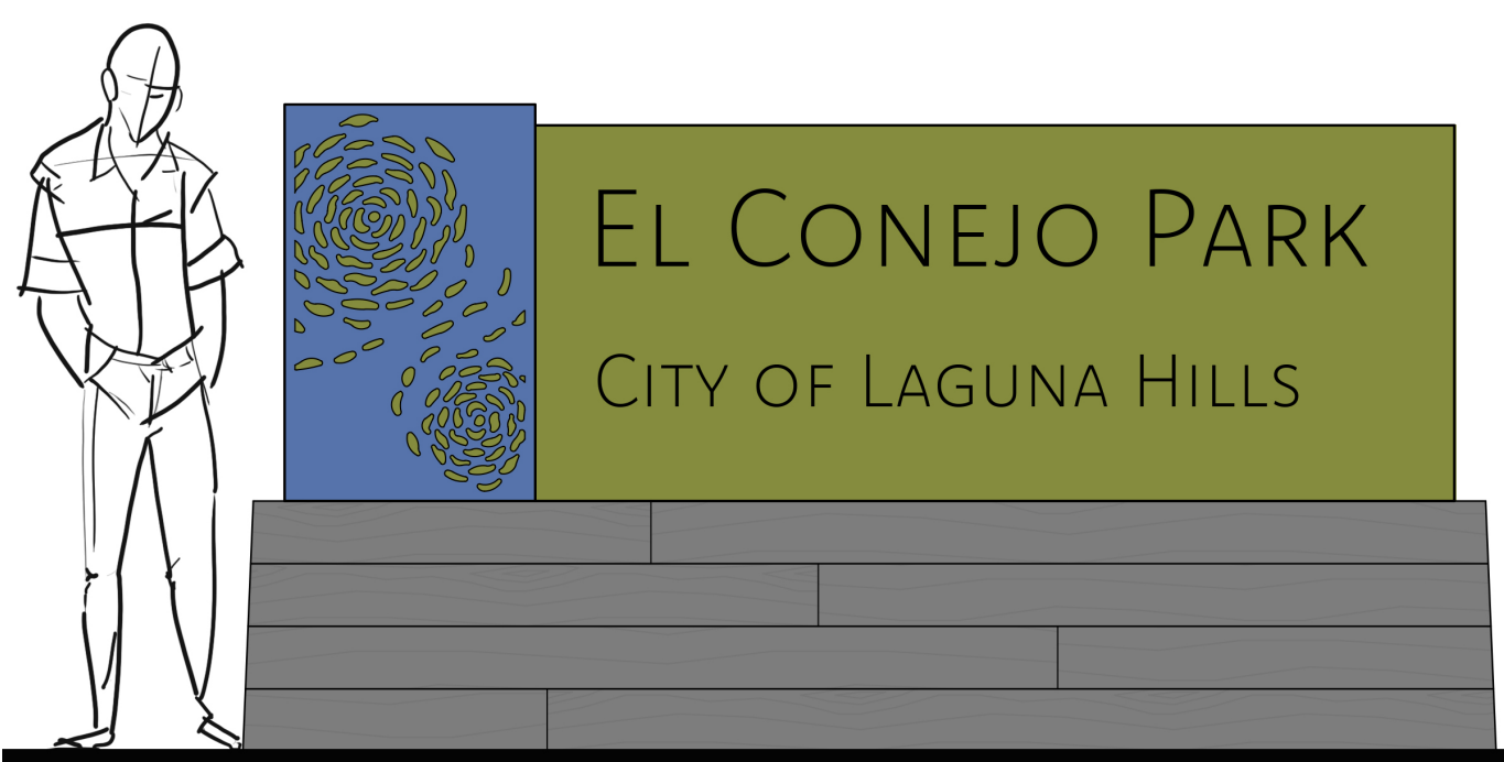
BOARDFORM CONCRETE BASE WITH CITY LOGO BRANDED COLOR METAL PANELING FOR LETTERS
