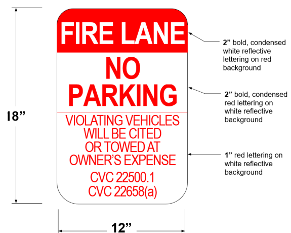
Figure 5 – Fire Lane No Parking Signs
