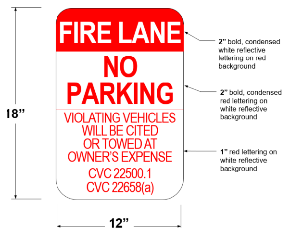
Figure 5 – Fire Lane No Parking Signs
