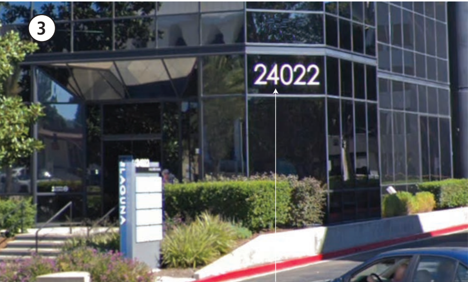
ADDRESS NUMERALS: EXISTING NON-ILLUMINATED FCO PVC ADDRESS NUMERALS @ FRONT ELEVATION. SIGN AREA = 10.53 SF.
